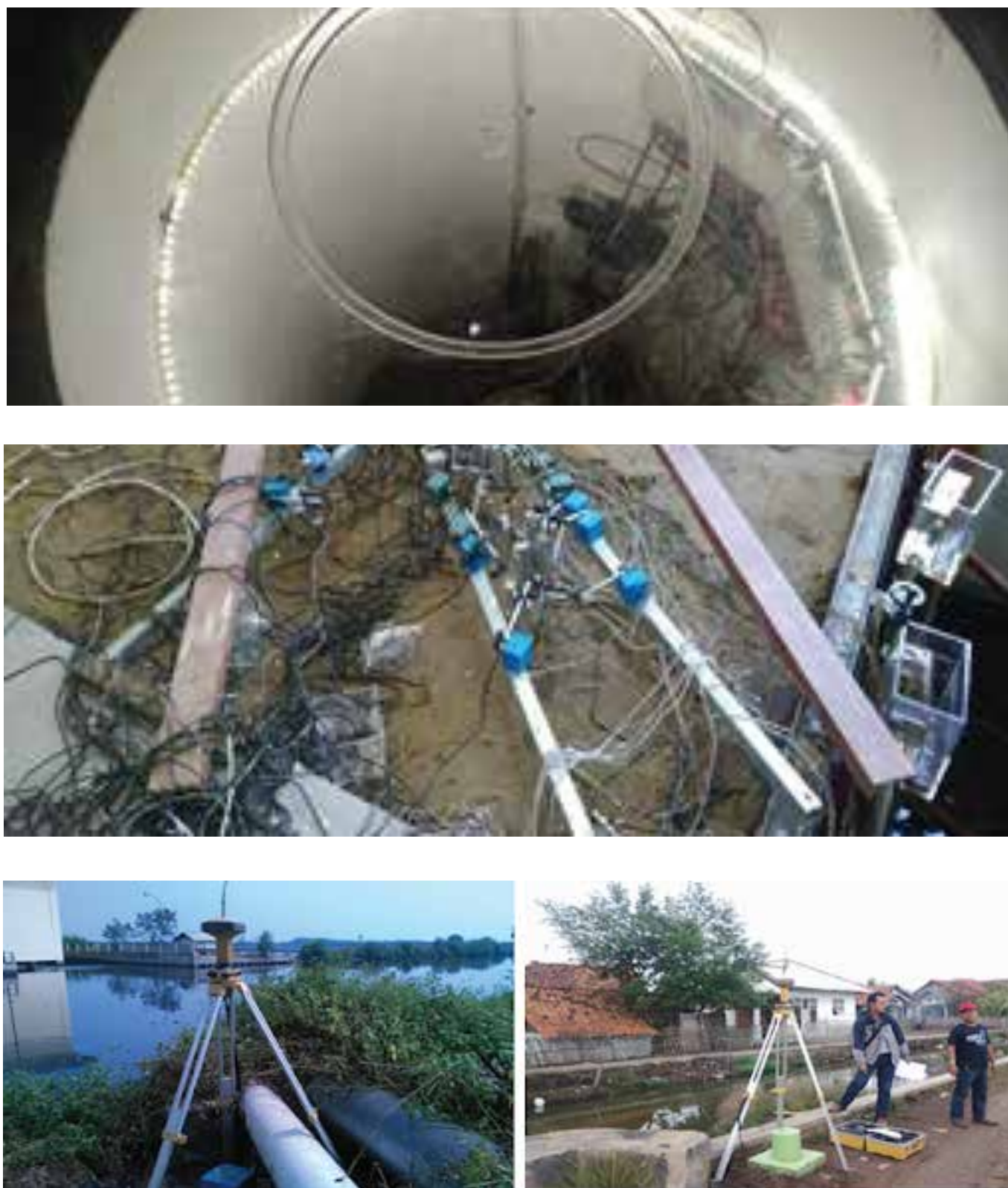
Figure 26. Documentation of land subsidence monitoring operation using GNSS in the northern coast of Java and land subsidence monitoring device in the city of Shanghai.
