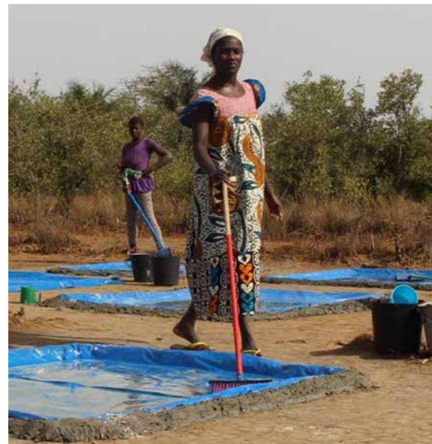
A new approach to salt production that makes use of solar heat instead of fuel wood was introduced in Guinea-Bissau – saving 3.1 kilos of wood per kilo of salt produced and reducing mangrove loss significantly.
