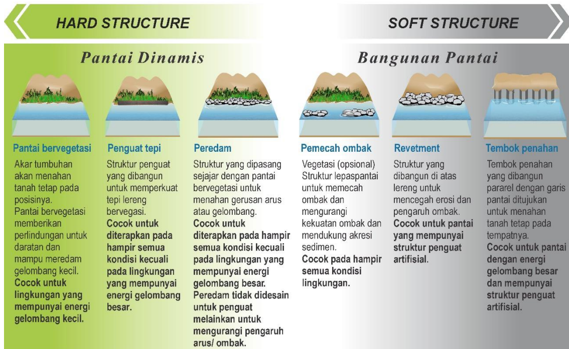
Gambar 3. Gambar skematis teknik stabilisasi garis pantai ( https://coast.noaa.gov/data/digitalcoast/pdf/living-shoreline.pdf )
