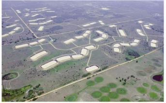
Figure 9 Rapid infiltration basins, Orlando, Florida (USGS
