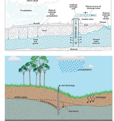
confining unit Figure 1 Artificial recharge of aquifers (USGS)
