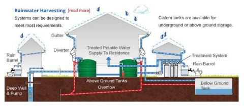
Figure 7 Rainwater Harvesting (Greenhouse engineering)
