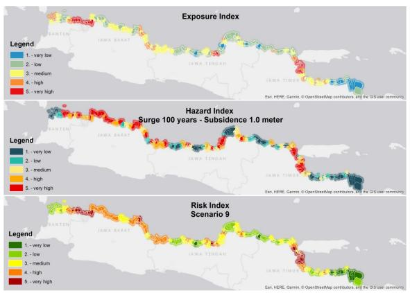
Figure 3.3 Risk of the north coast of java. The top plot shows the exposure index, the centre panel shows the hazard index for scenario 7 (SLR 0.06m, subsidence of 1.0m, surge with a return period of 100 year). The risk index (bottom panel) combines both the exposure and hazard index. Large numbers (red) indicate a large exposure, hazard and/or risk.
