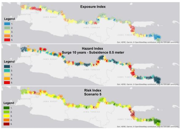
Figure B.5 Risk of the north coast of java. The top plot shows the exposure index, the centre panel shows the hazard index for scenario 5 (SLR 0.06m, subsidence of 0.5m, surge with a return period of 10 year). The risk index (bottom panel) combines both the exposure and hazard index.
