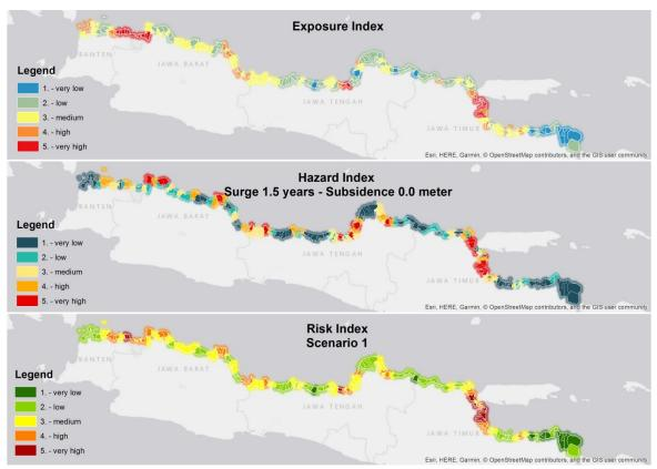
Figure 3.2 Risk of the north coast of java. The top plot shows the exposure index, the centre panel shows the hazard index for scenario 1 (SLR 0.06m, subsidence of 0.0m, surge with a return period of 1.5 year). The risk index (bottom panel) combines both the exposure and hazard index. Large numbers (red) indicate a large exposure, hazard and/or risk.
