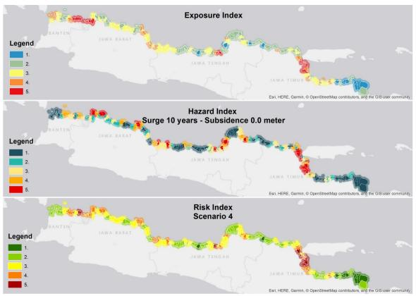
Figure B.4 Risk of the north coast of java. The top plot shows the exposure index, the centre panel shows the hazard index for scenario 4 (SLR 0.06m, subsidence of 0.0m, surge with a return period of 10 year). The risk index (bottom panel) combines both the exposure and hazard index.
