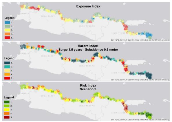
Figure B.2 . Risk of the north coast of java. The top plot shows the exposure index, the centre panel shows the hazard index for scenario 2 (SLR 0.06m, subsidence of 0.5m, surge with a return period of 1.5 year). The risk index (bottom panel) combines both the exposure and hazard index.
