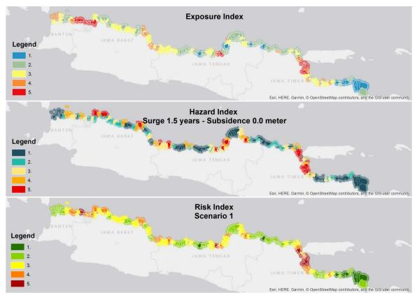
Figure B.1 Risk of the north coast of java. The top plot shows the exposure index, the centre panel shows the hazard index for scenario 1 (SLR 0.06m, subsidence of 0.0m, surge with a return period of 1.5 year). The risk index (bottom panel) combines both the exposure and hazard index
