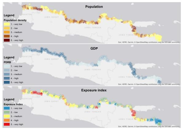
Figure 3.1 Exposure (bottom panel) of the north coast of Java, expressed using population density (top panel) and GDP (middle panel). Large numbers indicate a large population, GDP and/or exposure.
