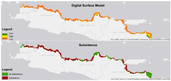
Figure 2.2 DSM (top panel) of the north coast of Java with high and relative safe areas in red/orange and low relative unsafe areas in yellow/green; and areas were subsidence occurs, derived from geological maps (bottom panel).
