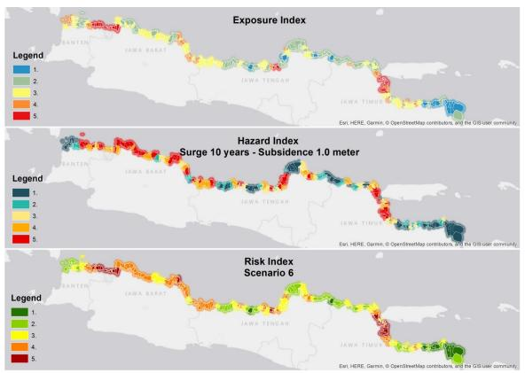
Figure B.6 Risk of the north coast of java. The top plot shows the exposure index, the centre panel shows the hazard index for scenario 6 (SLR 0.06m, subsidence of 1.0m, surge with a return period of 10 year). The risk index (bottom panel) combines both the exposure and hazard index.
