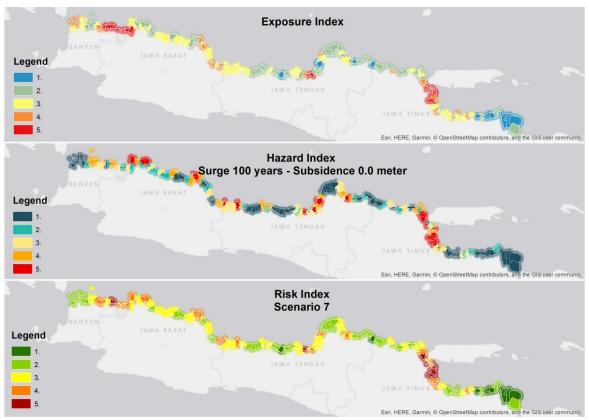
Figure B.7 . Risk of the north coast of java. The top plot shows the exposure index, the centre panel shows the hazard index for scenario 7 (SLR 0.06m, subsidence of 0.0m, surge with a return period of 100 year). The risk index (bottom panel) combines both the exposure and hazard index.
