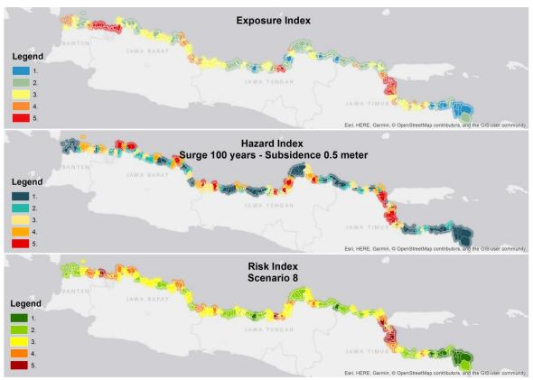
*Figure B.8* . Risk of the north coast of java. The top plot shows the exposure index, the centre panel shows the hazard index for scenario 8 (SLR 0.06m, subsidence of 0.5m, surge with a return period of 100 year). The risk index (bottom panel) combines both the exposure and hazard index.
