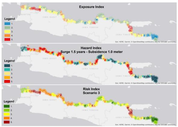
Figure B.3 Risk of the north coast of java. The top plot shows the exposure index, the centre panel shows the hazard index for scenario 3 (SLR 0.06m, subsidence of 1.0m, surge with a return period of 1.5 year). The risk index (bottom panel) combines both the exposure and hazard index.
