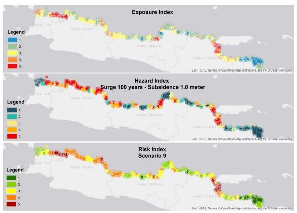
*Figure B.9*. Risk of the north coast of java. The top plot shows the exposure index, the centre panel shows the hazard index for scenario 7 (SLR 0.06m, subsidence of 1.0m, surge with a return period of 100 year). The risk index (bottom panel) combines both the exposure and hazard index.
