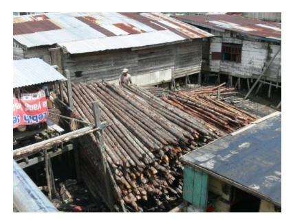
Figure 5. Bruguiera and Rhizophora poles taken from Bulungan mangrove forest, East Kalimantan, for construction works (Photo: Ilman, 2009)
