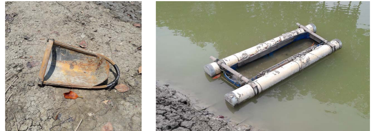
Figure 11: Shovel and raft used to dredge the pond and collect sediment to build the dyke (© Roel Bosma)
