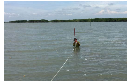
Figure 16. Measurement of level of stiff soil layer © Bagus Maulana
