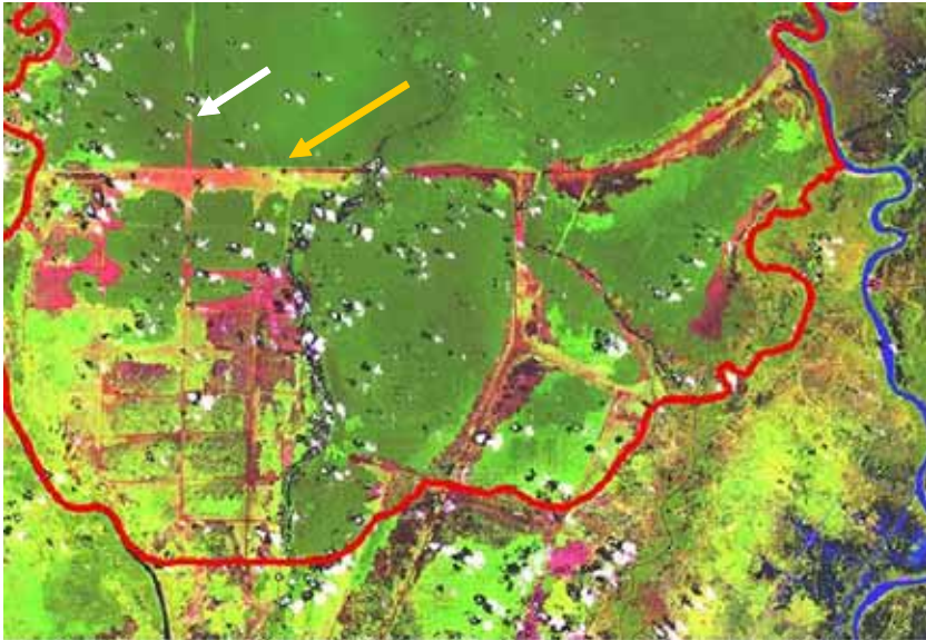
Illustration 4. Satellite image showing the location of a primary canal (white arrow) and the main primary canal (yellow arrow) in Central Kalimantan
